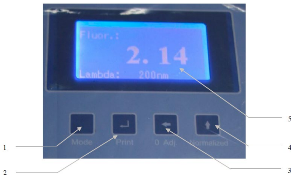
1. Mode key, 2. Print key, 3. Adj 0% key, 4. Normalize key, 5. Display Window.
