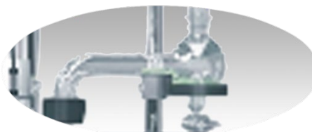
Pumping and filling nozzle
